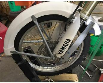
Here is a front fender mount design for Upside Down forks contributed by Mike Bauer, one of my summer & winter riding friends. Notice the triangulated forward struts to defend against impact and they have a hollow construction to reduce side-to-side fender wiggle—basically so the studs don't chew up the fender.
