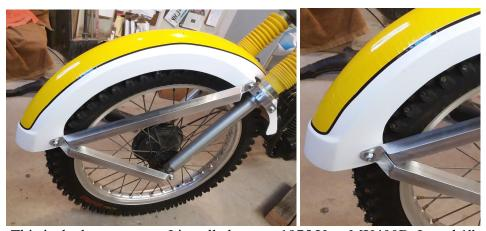
This is the brace system I installed on my 1975 Yam MX400B. I used 1" square box aluminum tubing. Angle cut ends for screw access. Clumsy looking but it works
